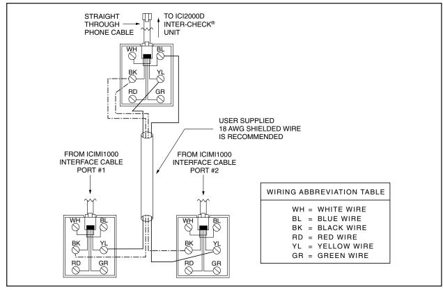
Figure 2. Wiring Diagram for Two Cash Registers or Two ATM Machines
